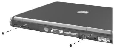
Removing the Display Assembly Screws
